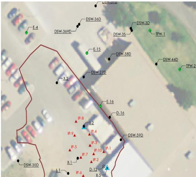
Figure 1 indicates the layout of direct push injection points depicted in red, EHC Liquid amendment injection wells depicted in blue, and the down gradient extraction wells in green.
