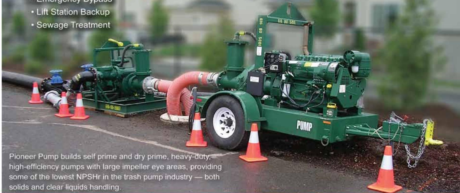
Pioneer Pump builds self prime and dry prime, heavy-duty, high-efficiency pumps with large impeller eye areas, providing some of the lowest NPSHr in the trash pump industry — both solids and clear liquids handling.
